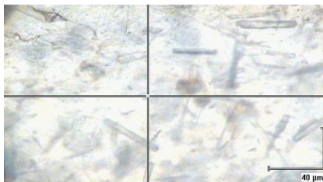
Figure 5 Optical micrograph of PE/EMA/wollastonite-ppy composite.
